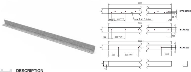
We offer shelf angles that are 3 meters long and can be purchased in bulk. These shelf angles come with predrilled 20mm holes at 300mm intervals, but we also offer customization options for hole spacing and drill patterns.
